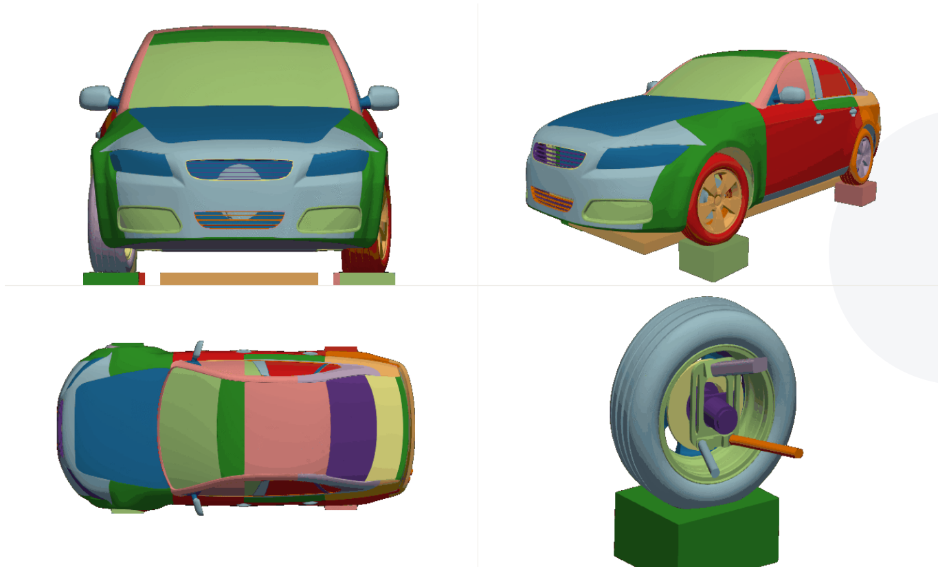
Sweep geometry studies: car positioning, wheel steering and surface morphing boxes through DoE
