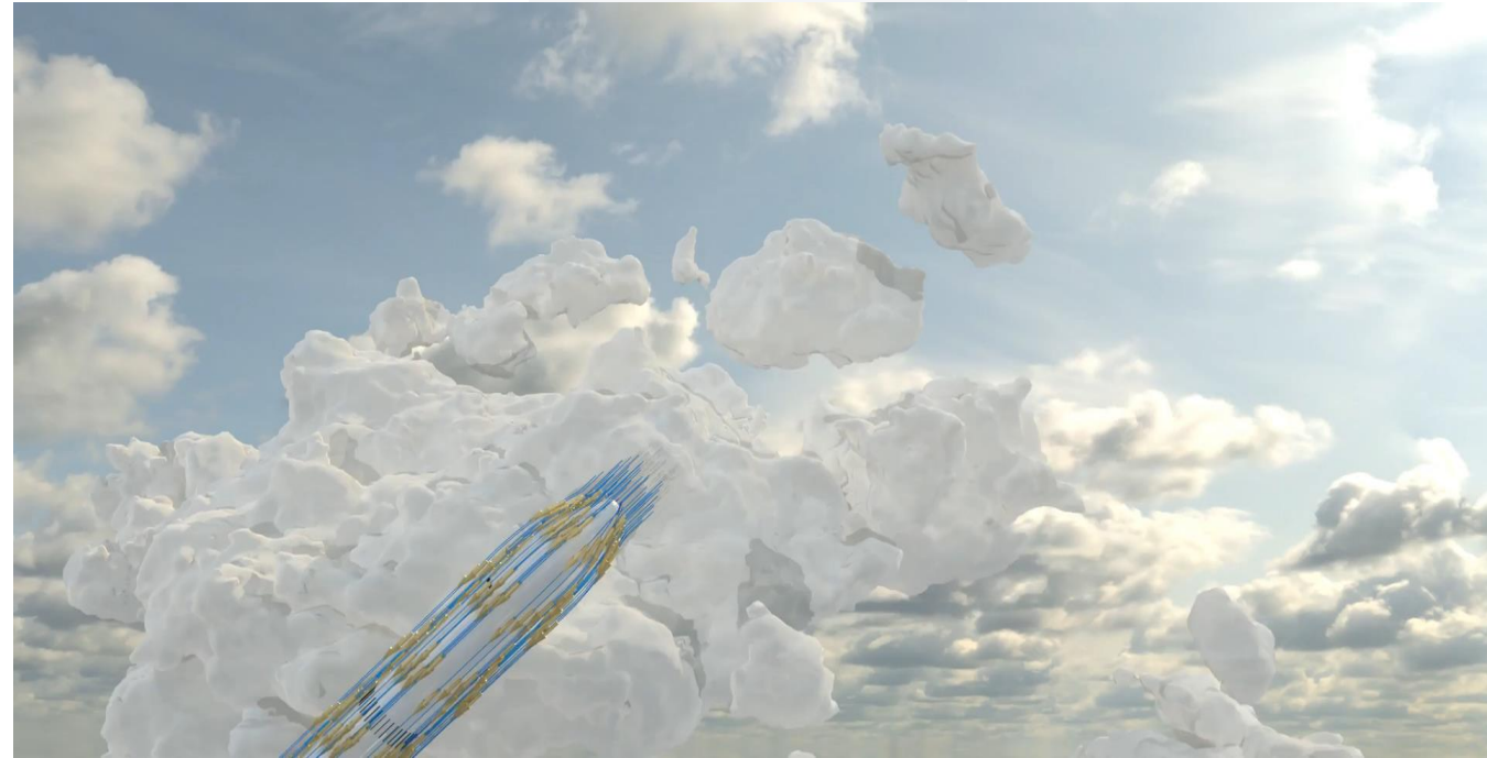
MaiaSpace reusable launcher, ~50m cells, RANS, M=2, iconCFD V5
