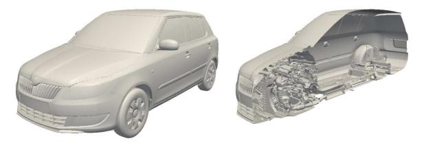
Figure 18: Wrap and clip through wrapped surface of UTHM model
